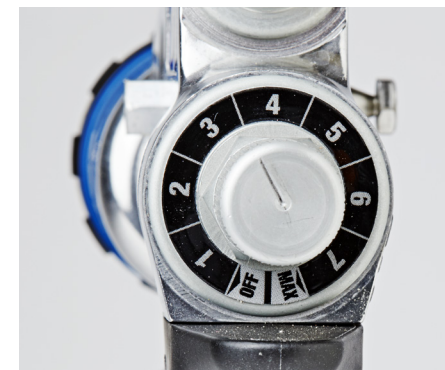
Graco's gun has an intuitive finish adjuster: The higher the number, the more finish flows into the airstream.
